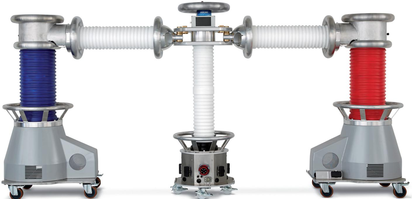
The high power HVA200 Test System is capable of testing cables up to 141 kV (Test Voltage 1.7 x U0). The smallest and lightest VLF unit of his class offers VLF (Very Low Frequency) 0.1 Hz standard testing as well as DC output voltage up to 200 kV. The HVA200 system can be upgraded with optional Tan Delta or Partial Discharge Diagnostics Systems. This space saving configuration allows the test set to be mounted on a van or trailer or can be transported in solid transport boxes (optional).
