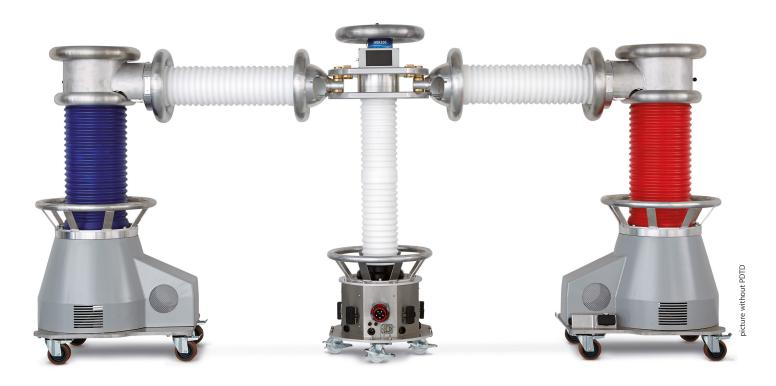
The high power HVA200 Test System is capable of testing cables up to 140 kV (Test Voltage 1,7 x U0) and allows to diagnose these cables with Partial Discharge and Tan Delta Diagnostics. The HVA200 is for laboratory use or can be fitted as a mobile test laboratory into a van. The smallest and lighvtest VLF unit of his class offers VLF (Very Low Frequency) 0.1 Hz standard testing as well as DC output voltage up to 200 kV.
