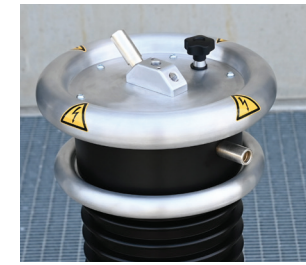
Top view: HV connections
